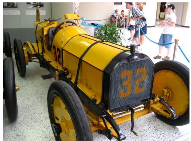
Ray Harroun's Wasp, winner of the 1911 Indianapolis 500. The car's rear-view mirror is mounted on struts ahead of the steering wheel.
